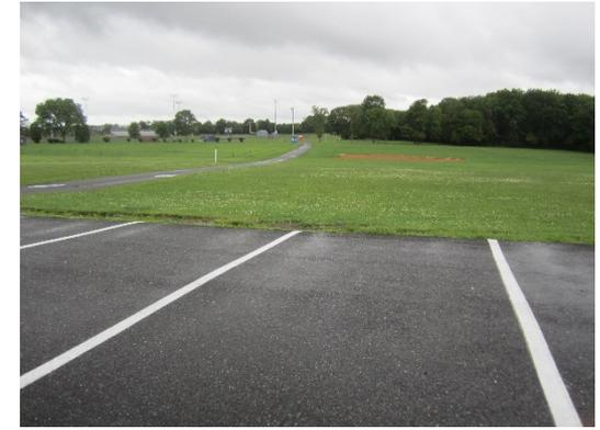
A section of parking spaces can be converted to porous pavement to capture and infiltrate runoff from the parking lot. Overflow runoff can be treated with a rain garden installed in the turfgrass area adjacent to the pervious pavement. A preliminary soil assessment suggests that more soil testing would be required before determining the soil's suitability for green infrastructure.
